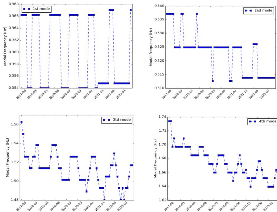
**Fig. 6.** Monthly average natural frequencies of a high-rise building for first 4 modes, and for 66 months under ambient vibration
