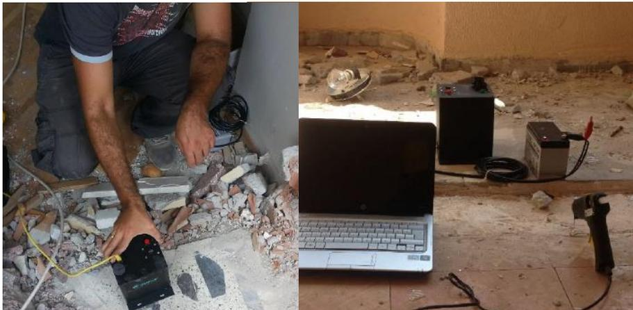
**Fig. 3.** Ultra-sensitive eQUAKE acceleration recorder glued to the rigid floor area at 6<sup>th</sup> floor and exactly to the same location in both buildings
