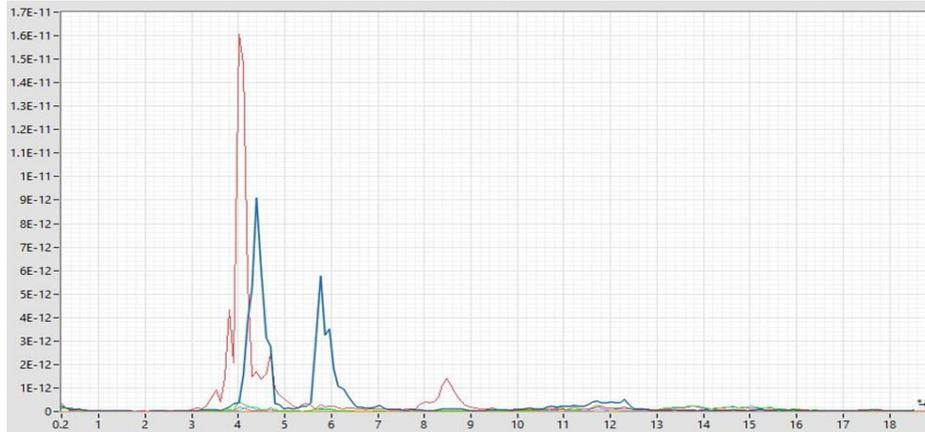
**Fig. 10.** PSD graph, natural frequencies corresponding to first 4 bending modes of the building
