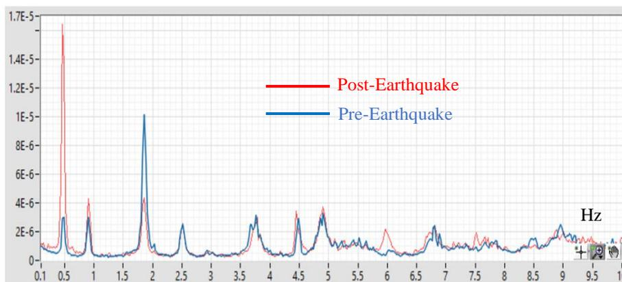
**Fig. 5.** Before and after comparison. Natural frequencies of the high-rise building (Fast Fourier Transform of the Recorded Acceleration under ambient vibration)
