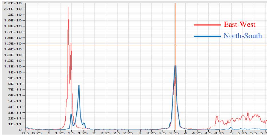
Fig. 8. PSD graph, natural frequencies corresponding to first 3 modes of the building
