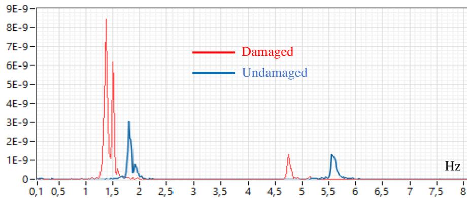
**Fig. 4.** 33% natural frequency shift in both 1<sup>st</sup> and 2<sup>nd</sup> modes due to induced damage (PSD of the Recorded Acceleration)
