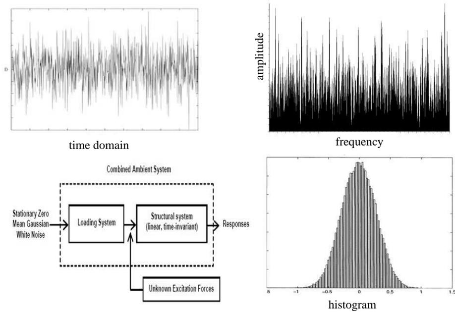
**Fig. 1.** White-noise, time/frequency domain, histogram, combined ambient system
